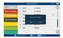
Select [Heater Mode] menu. Select [Delete Heat Mode]. Select the heat mode to be deleted
