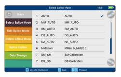
Selected splice mode appears on the screen. Press [Reset] button to return to the initial interface page.
