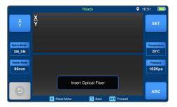
Selected heat mode appears on the screen. Press [R] button to return to the initial interface.
